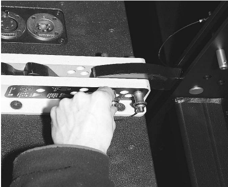
Fig. 28: Splay link of the frame connected to the first cabinet
