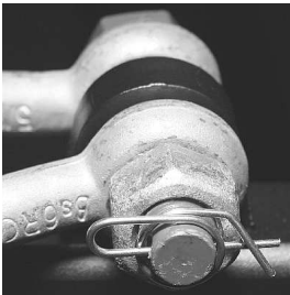
Fig. 22: Ring cotter to secure the 3.25 t shackle [S].
